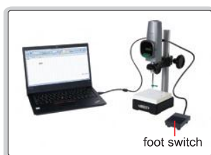
data transmitted to Excel without software; short press the foot switch to transmit data, long press to zero
